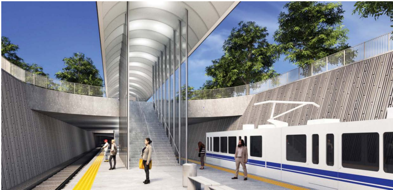
Figure 6 - Trenched Grade Separation with Station
